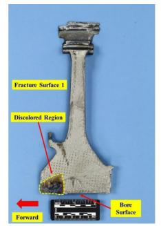
Failure Surface of the High Pressure Turbine Stage 2 Disk from AA383
