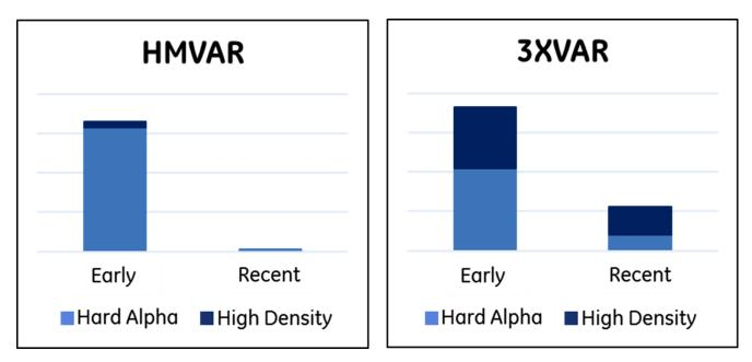
Figure 6: Premium Quality Ti hard-alpha and high-density inclusion rates for HMVAR and Triple-VAR (5)
