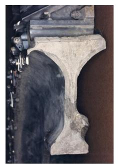
Failure Surface of the Stage 1 Fan Disk from UA232
