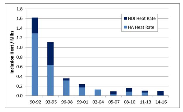
Figure 5: Hard-alpha and high-density inclusion rates from 1990 through 2016 in Premium Quality Ti (5)
