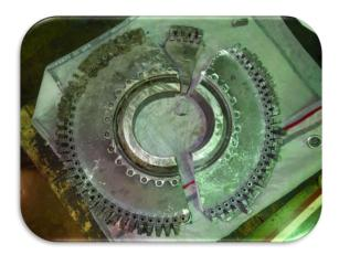
Recovered fragments of the High Pressure Turbine Stage 2 Disk from AA383
